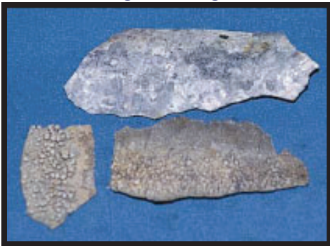
2B Curved scale chips that broke away from a large diameter pipe.
