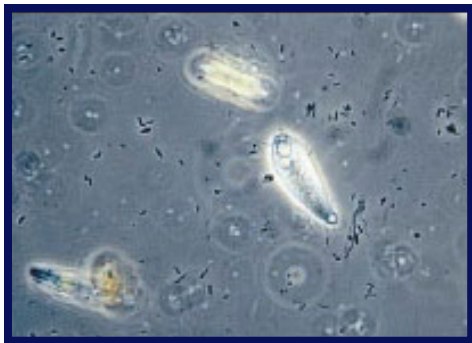
4B A variety of rod-shaped bacteria and two protozoans found in a recirculating cooling system.
